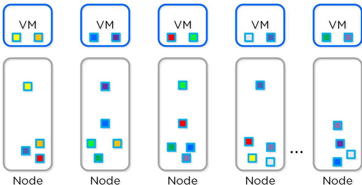
Figure 8: Typical Replication Factor Data Layout
