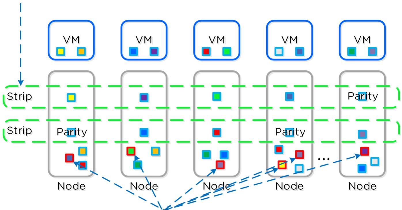
Once the strip and parity has been calculated the replica extent groups can be removed, providing the storage savings
